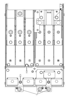
Illustration 5.64 1) Position of Earth Terminals IP20 (chassis), D-Frame Sizes
