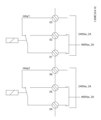
Illustration 5.100 D-frame Additional Relay Outputs
