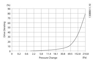
Illustration 5.26 E-Frame Derating vs. Pressure Change (Large Fan), P315T5-P400T5 and P500T7-P560T7 Frequency Converter Air Flow: 850 cfm (1,445 m<sup>3</sup>/h)
