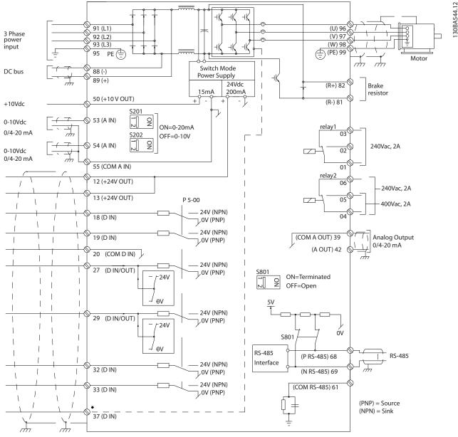
Illustration 5.53 Interconnect Diagram E-frames and F-frame (6-pulse)
