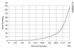
Illustration 5.24 D-Frame Derating vs. Pressure Change Frequency Converter Air Flow: 450 cfm (765 m<sup>3</sup>/h)
