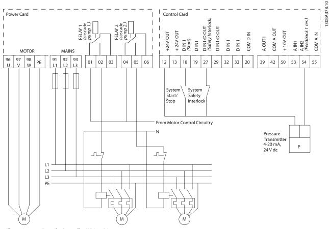
Illustration 6.9 Cascade Controller Wiring Diagram
