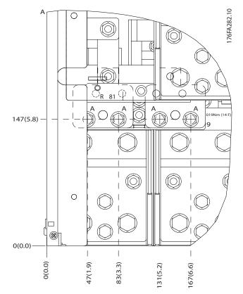
Illustration 5.80 IP00 Enclosure Power Connection Positions
