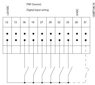
Illustration 5.57 Input Polarity of Control Terminals
