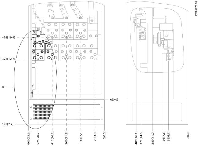
Illustration 5.76 IP21 (NEMA Type 1) and IP54 (NEMA Type 12) Enclosure Power Connection Positions
