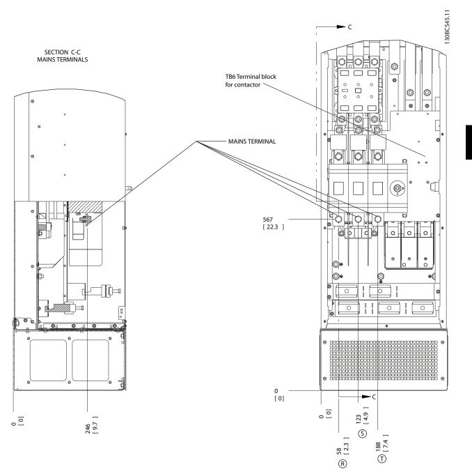
Illustration 5.74 Terminal Locations, D8h with Contactor and Disconnect Options
