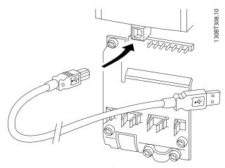
Illustration 5.105 Connection of PC to Frequency Converter
