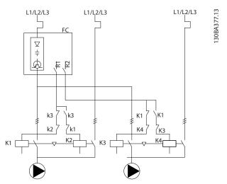
Illustration 6.11 Lead Pump Alternation Wiring Diagram
