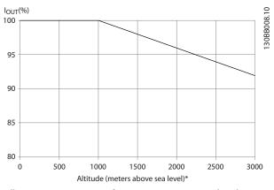
Illustration 3.3 Derating of Output Current Versus Altitude at  $T_{\text{AMB, MAX}}$
