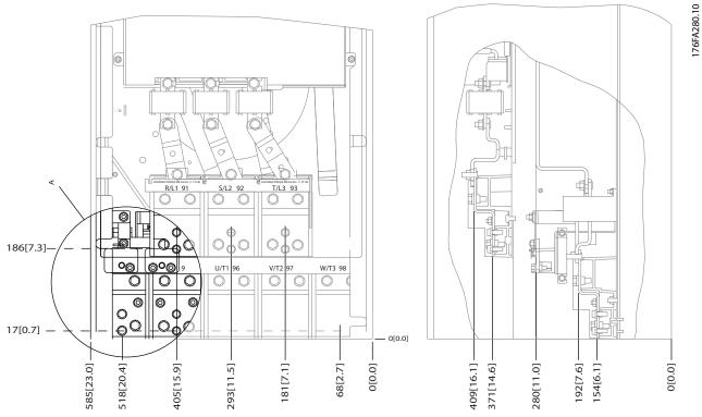
Illustration 5.79 IP00 Enclosure Power Connection Positions
