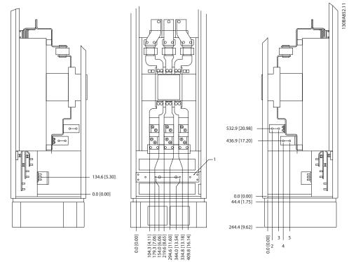
Illustration 5.89 Terminal Locations - Options Cabinet with Circuit Breaker/Molded Case Switch (Left, Front and Right Side View). The Gland Plate is 42 mm below .0 level.
