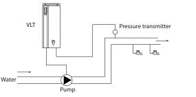
Illustration 2.16 Closed Loop PID Control
