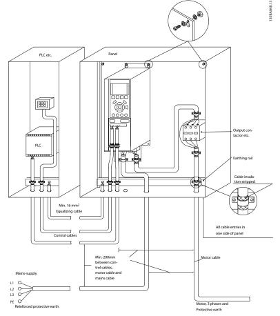
Illustration 5.106 EMC-correct Electrical Installation of a Frequency Converter in Cabinet
