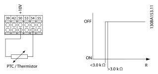
Illustration 2.30 Analog Input 10 V Power Supply
