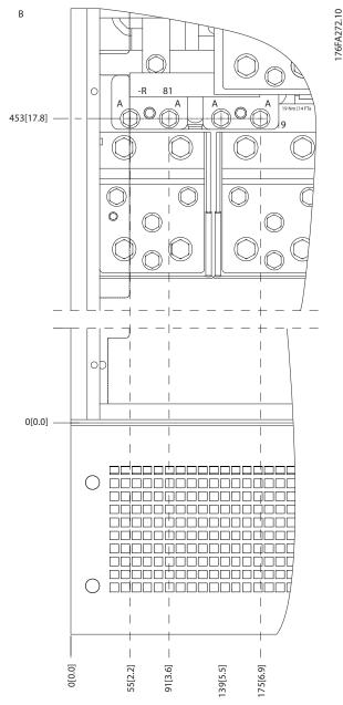
Illustration 5.77 IP21 (NEMA type 1) and IP54 (NEMA type 12) Enclosure Power Connection Positions (detail B)
