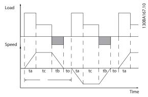
Illustration 2.25 Typical Braking Cycle
