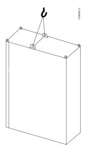
Illustration 5.8 Recommended Lifting Method, Frame Sizes F1, F2, F9 and F10
