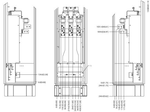
Illustration 5.88 Terminal Locations - Options Cabinet (Left, Front and Right Side View). The Gland Plate is 42 mm below .0 level. 1) Earth ground bar
