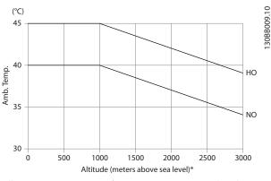
Illustration 3.4 Derating of Output Current Versus Altitude at TAMB, MAX
