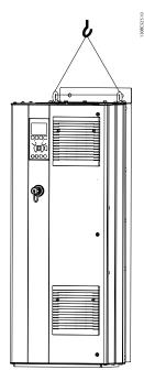
Illustration 5.6 Recommended Lifting Method, D-Frame Size
