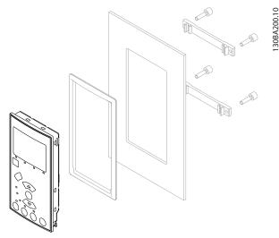
Illustration 3.18 LCP Kit with Numerical LCP, Fasteners, and Gasket.
