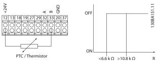
Illustration 2.28 Digital Input and 24 V Power Supply
