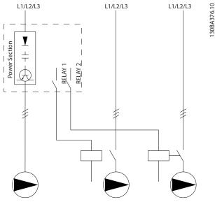
Illustration 6.10 Fixed Variable Speed Pump Wiring Diagram
