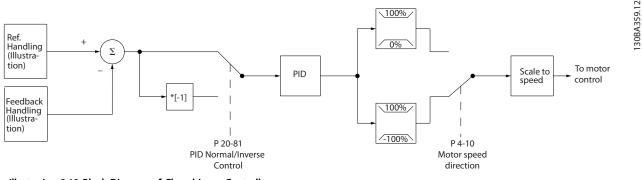
Illustration 2.12 Block Diagram of Closed Loop Controller
