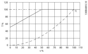
Illustration 3.5 Maximum Load for a Standard Motor at 40 °C
