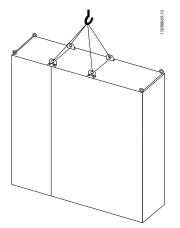
Illustration 5.9 Recommended Lifting Method, Frame Sizes F3, F4, F11, F12 and F13
