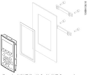
Illustration 3.17 LCP Kit with Graphical LCP, Fasteners, 3 m Cable, and Gasket. Ordering No. 130B1113
