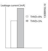
Illustration 2.22 Influence of Line Distortion on Leakage Current
