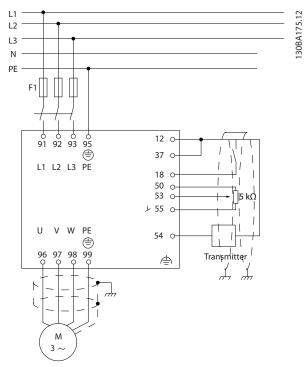
Illustration 5.107 Electrical Connection Diagram (6-pulse example shown)
