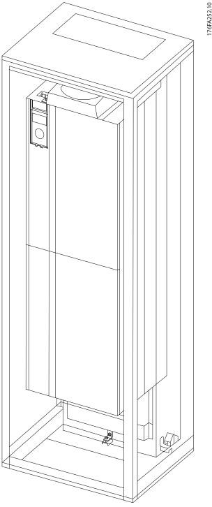
Illustration 3.19 Installation of IP00/IP20/Chassis in Rittal TS8 Enclosure.
