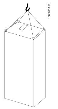
Illustration 5.10 Recommended Lifting Method, Frame Sizes F8
