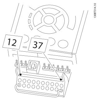
Illustration 5.102 Bridge Jumper between Terminal 37 and 24 V DC
