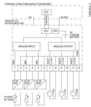
Illustration 3.11 Principle Diagram for Analog I/O Mounted in the Frequency Converter
