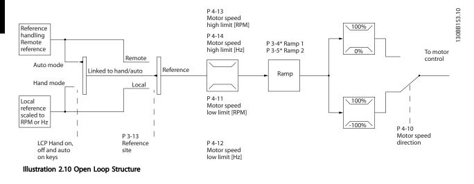
In the configuration shown in *Illustration 2.10, 1-00 Configuration Mode* is set to [0] Open loop. The resulting reference from the reference handling system or the local reference is received and fed through the ramp limitation and speed limitation before being sent to the motor control. The maximum frequency allowed limits the output from the motor control.
