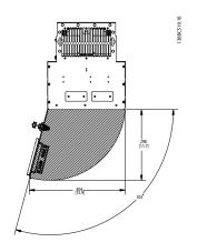
Illustration 5.11 Front Clearance of IP21/IP54 Enclosure Type, Frame Size D1h, D5h, and D6h.
