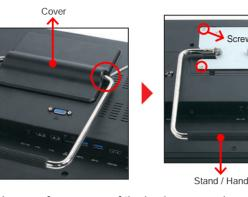
2. Unscrew four screws of the back cover and remove it.
