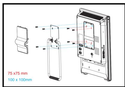
■ If you are mounting your X50V6 to the wall, remove the cover on the back of
