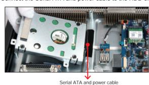
4. Install the HDD or SSD & bracket in the chassis and tighten the HDD or SSD & bracket with four screws.
