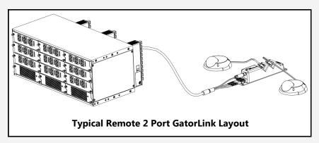
**Stand Alone 2 Port SFP GatorLinks** operate in a similar manner to Remote units except, they come with their own dedicated power supply which is used to provide power to the GatorLink using local power. These devices can be placed anywhere that local power is accessible.
