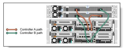
Figure 9. DM7100F NVMe expansion connectivity topology: One enclosure
