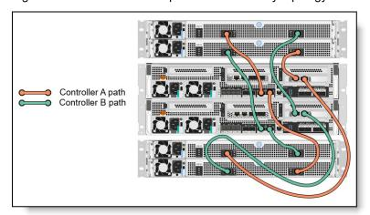
Figure 10. DM7100F NVMe expansion connectivity topology: Two enclosures
