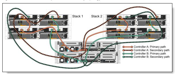
Figure 12. DM7100F SAS expansion connectivity topology: Two stacks
