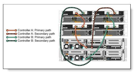
Figure 11. DM7100F SAS expansion connectivity topology: One stack
