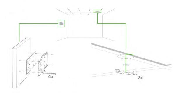
1. Attach the T-rail clips to the T-rail by rotating them and snapping them into place as shown. The black foam pads should be compressed slightly after installation.
