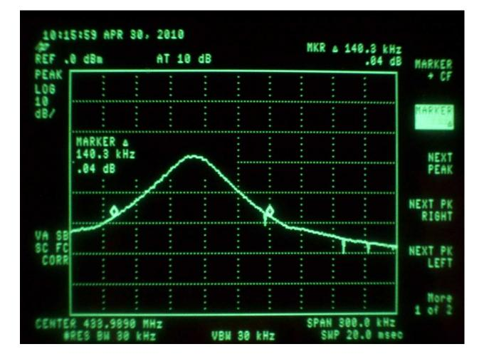
Bandwidth of the modulated signal is 140 kHz
