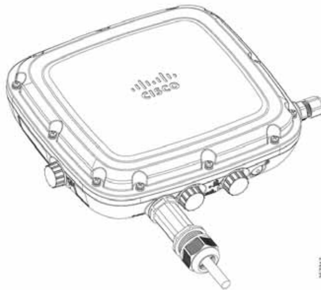
Figure 53: Fiber-Optic cable and gland installed to AP
