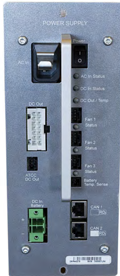
Figure 184: Power Supply Unit Front Panel
