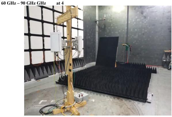
Radiated Emissions 90 GHz – 100 GHz at 4
