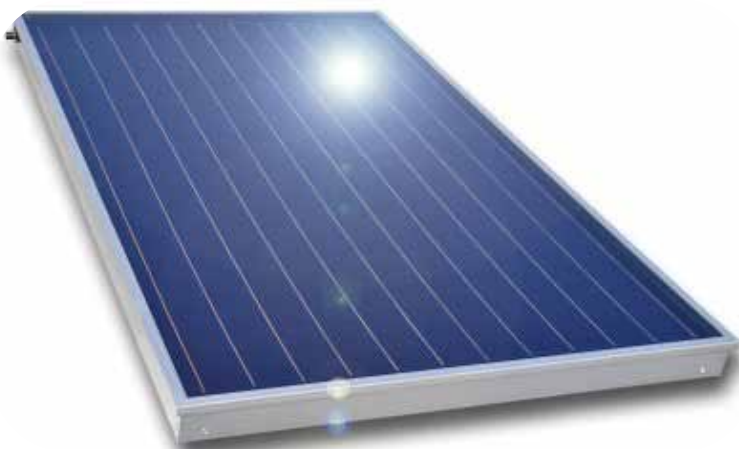
Figure 3.13. Flat plate collector with selective coating on the absorber. The parallel lines indicate where the riser tubes are connected to the absorber by ultra-sonic welding.
