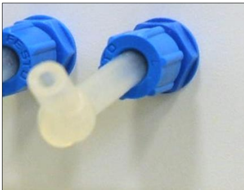
Figure 14: Knotted tubings to secure the fluid connections
