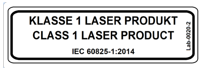
Figure 2: Class 1 Laser Product label
