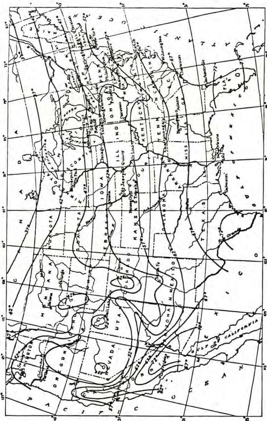
(From Collins, W. D., U.S. Geol. Survey, Water-Supply Paper 520-F.) Figure 38. Approximate temperature of water from nonthermal wells at depths of 30 to 60 feet.
