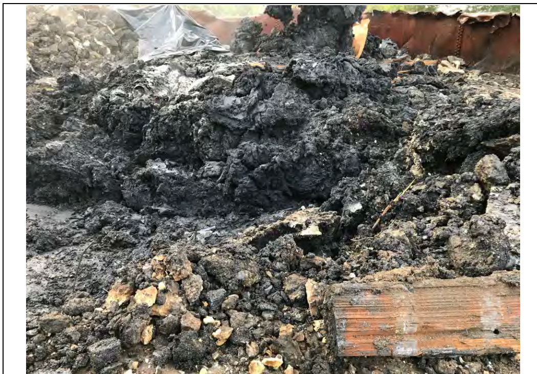
Date: 09/22/2017 Site Name: Troy (Water Street) Site - Area 3 Photographer's Initials: JAJ Description: Photograph #14: Tar-impacted fill/debris found beneath concrete within Former Tank T-41.
