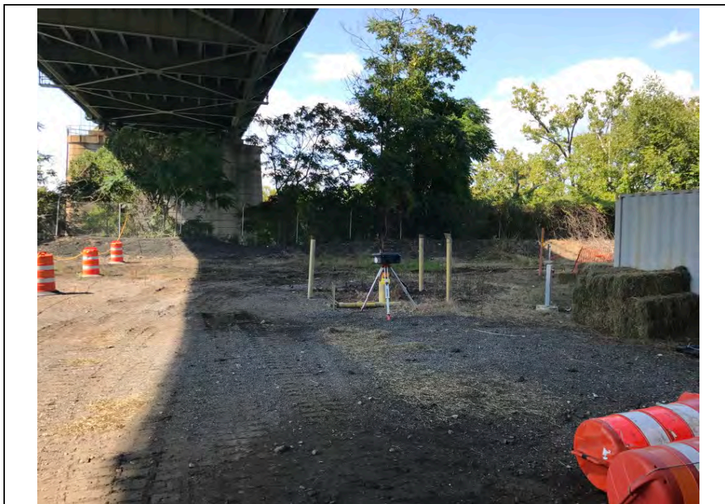
Date: 09/19/2017 Site Name: Troy (Water Street) Site - Area 3 Photographer's Initials: JAJ Description: Photograph #2: Installed perimeter air monitoring station (center) and temporary barricades (left). Photograph taken facing West.
