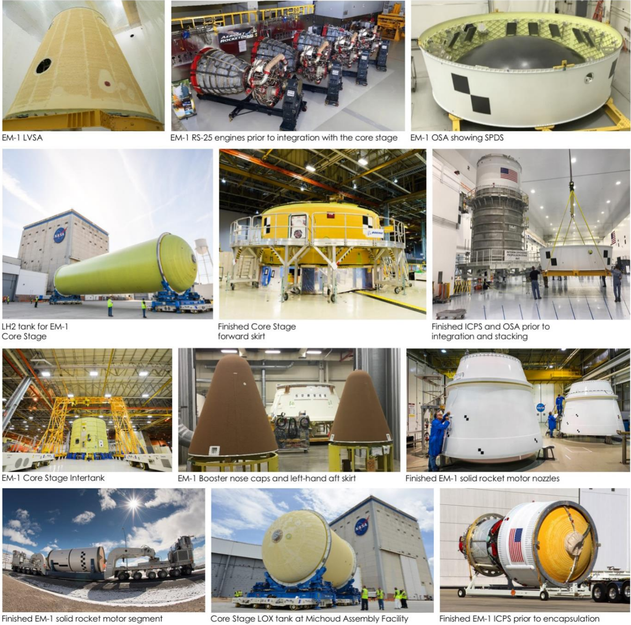
Figure 3-11. SLS Block 1 Progress in Support of First Flight (EM-1)
