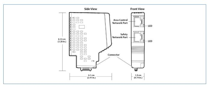
SZ Controller Ethernet Isolation Port or Keylock Ethernet Isolation Port.
