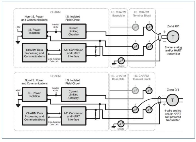
Simplified Circuit and Connection Diagrams for LS IS AI-CHARM 4 to 20 mA HART Two-Wire and Four-Wire transmitters.
