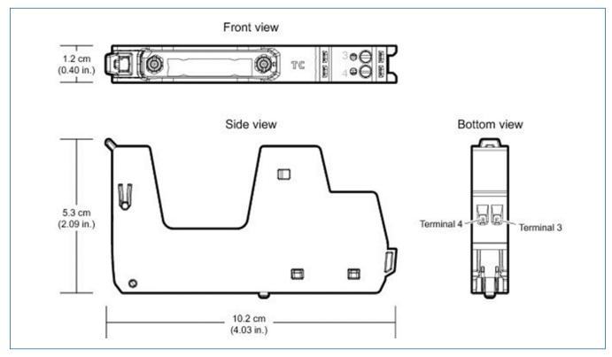
IS CHARM Thermocouple / mV Terminal Block.
