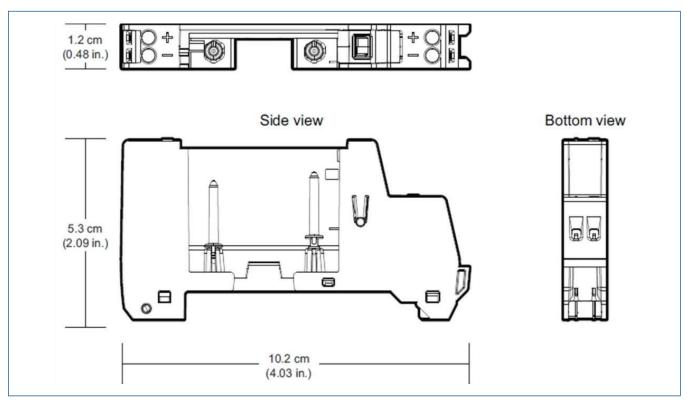
Address Plug Terminal Block for IS Baseplate.
