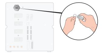
3 Use a 4 mm Allen key to remove the four screws holding the Venturi pump.
