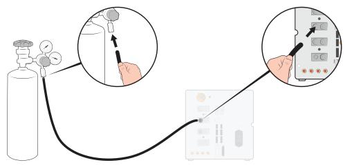
6 Open cylinder valve and set regulator to desired pressure. See warning banner!
