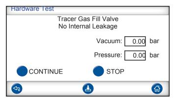
The step tests the gas fill valve for internal leakage by registering pressure rise behind the valve.
