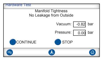
The overall tightness of the manifold is tested using the vacuum raise method. Possible results:
