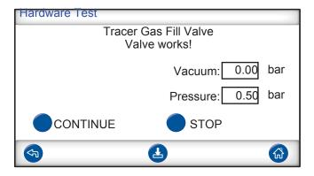
This step tests that tracer gas fill valve opens to fill gas. Test will fail if tracer gas feed pressure is too low. If this is the case, adjust pressure and restart hardware test from beginning.
