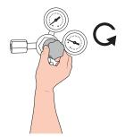
**5** Connect a regular welding gas hose or similar between the Tracer Gas Port and the pressure regulator. Check that the hose is certified to withstand the maximum output pressure of the regulator.
