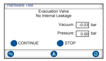
Evacuation valve is checked for internal leakage. Possible results:
