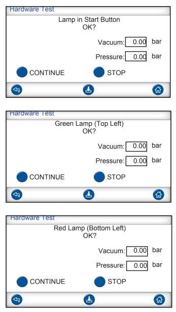
This is a "manual" test. The ILS500 lights up one lamp at the time. Simply check that the right lamp comes on.
