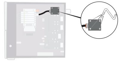
4 Remove the o-ring under the Venturi. Remove the hose from Venturi inlet.
