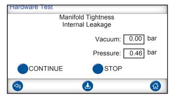
The overall tightness of the manifold is tested using the pressure decay method. This is a complement to the gas test, revealing leakage out, through the exhaust etc. Possible results:
