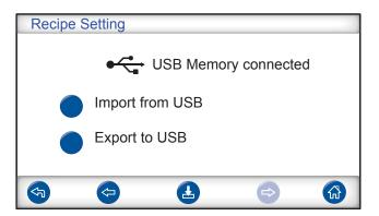
An icon for USB is shown when installing the USB flash drive.
