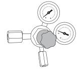
4 Turn regulator fully counter clockwise for zero output pressure.
