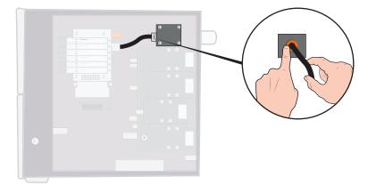
**5** Remove the hose fitting from the Venturi.
