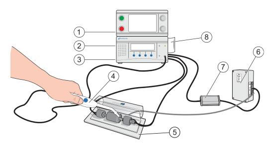
Chamber Test with Leak Locating Option
