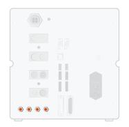
Tooling Valve Outputs 1-4 is available for connection of external Tooling. If the test object has 2 or more ports, connect to ports on opposite sides of object.
