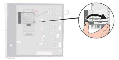
4 Push the screw in while inserting the new valve. Insert the end facing the screw first and then push the coil side down.
