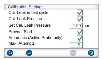
Calibration Value Calibration Unit Leak Gas Set to the same as stated on the calibration certificate issued for the leak or gas. Set to the same as stated on the calibration certificate issued for the leak or gas. Set the gas flow for which the Calibration Leak is defined.
