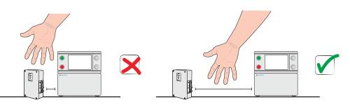
Some free space must be provided around the ILS500 to enable maintenance and service access.
