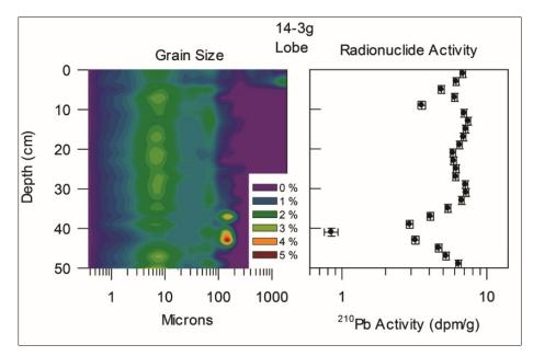
Figure 39. Grainsize and <sup>210</sup>Pb in core 14-3g
