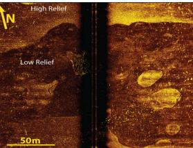
**CP10.12 8** Sidescan sonar image showing the lower part of a large mudflow deposit with prominent scarping.
