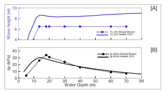
Figure 43. Wave forcing on seabed
