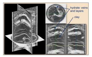
Figure 66. 3D x-ray in pressurized core
