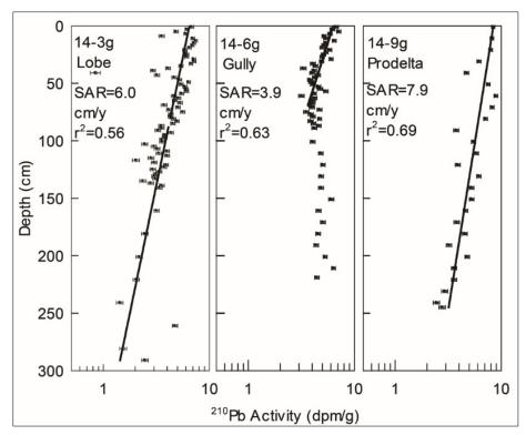
Figure 39. <sup>210</sup>Pb profiles for gravity cores
