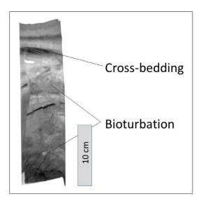
Figure 13. X-radiograph of gully core
