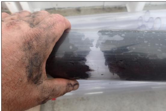
**Figure 65. Gas expansion in core.**
