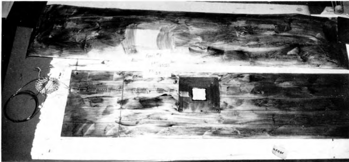
Figure 11. Contact cement on aluminum and PVC laminate.
