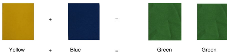
FIGURE 6 Subtractive colour mixing of yellow and blue SC-CO 2 dyed polyester fabrics to produce two uniformly coloured green fabrics.
