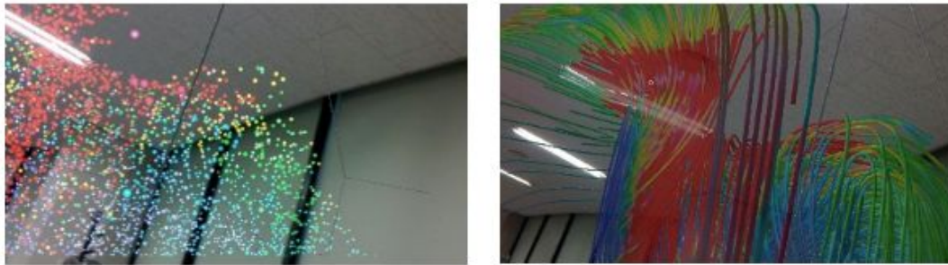
Figure 2: Kim et. al., 2018’s simulation of real-time aerodynamic flow simulation from an air purifier. The results were generated using a high-performance compute node, and downloaded and visualised in real-time using the Unity game engine. The authors praised the visualisation for allowing them the review CFD results accurately.
