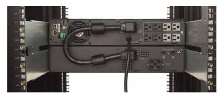
A UPS paired with an extended battery module helps extend runtime to meet service level agreements.
