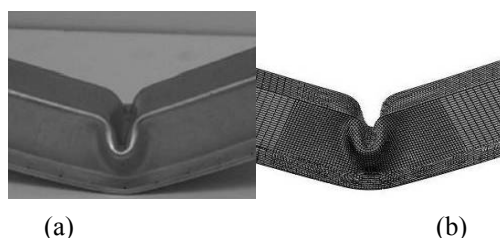
Figure 11. Comparison of collapse modes of a closed-hat-section beam from (a) existing experiment and (b) present remodel
