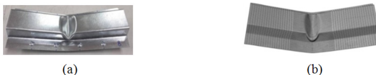
Figure 16. Comparison of collapse mode of closed-hat-section beam between (a) experiment and (b) present simulation
