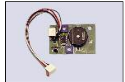
PASSING CHIME BOARD Part #: 70B09P02 Model: MPCB-1 to be used with Digital Position Indicators
