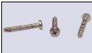
4X3/4 (PZ) #4 x 3/4" Phillips Pan HD Thread Forming Mtl: Zinc Plated (Sheet Metal Screw)
