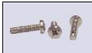
8-32X3/4 (PZ) #8-32 x 3/4" Phillips Pan HD Thread Forming Mtl: Zinc Plated
