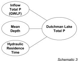
Schematic 3 BATHTUB Model Schematic.
