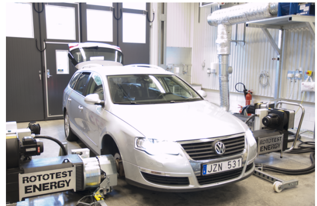
Figure 2. Vehicle mounted at Vehicular Systems chassis dynamometer laboratory at LiU.
