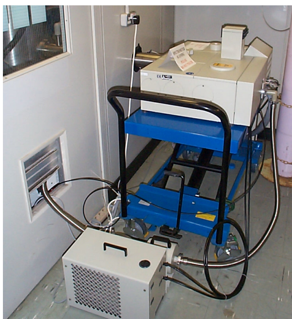
Figure 4.6: The Bruker IFS 66v/S spectrometer, sited inside the air-conditioned spectrometer room at the MSF, connected by an evacuated tube to the large aerosol cell visible through the window.
