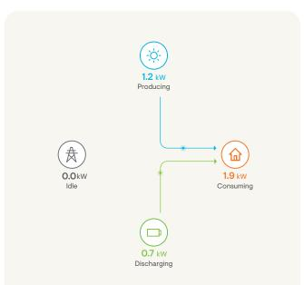
During peak hours, if the export tariff is less than the import tariff, power export is not profitable. Solar production and the battery power the home, minimising power import from the grid.
