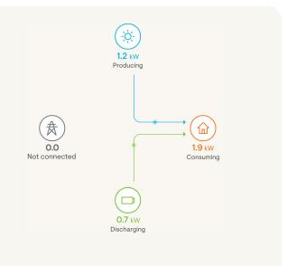
When the grid is down, solar and battery power the home.
