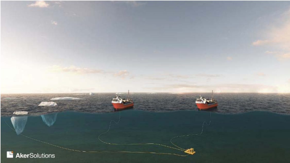
Figure 1-1 Power from shore utilizing a subsea transformer for voltage stepdown and power distribution
