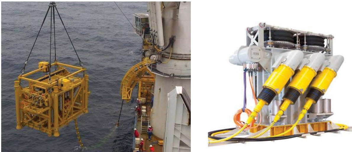
Figure 8-20: 19 MVA Aker Solutions Åsgard subsea compressor transformer module (left) and ABB subsea transformer unit (left). The Mecon 145kV Dry Mate connection is shown with yellow paint.
