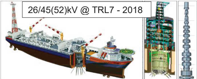
Figure 9-1: Position-anchored production ship with geostationary swivel tower – ref. SBM / Equinor
