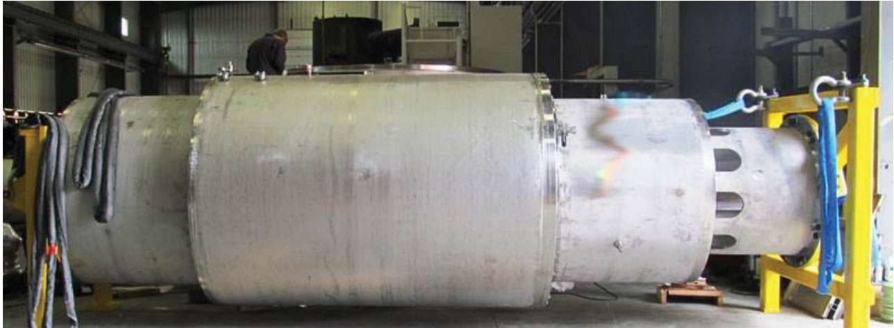
Figure -: BZ-25 MVES – Ex o, IP66, 9 × 35kV @ 400A sliprings, approximately 8.5m tall – Focal
