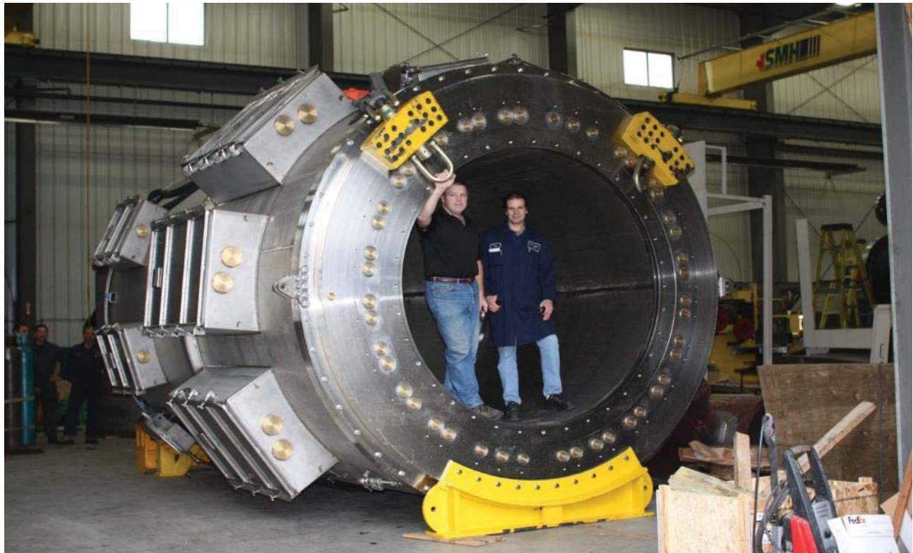
Figure 8-28: OSX-3 MVES, Exp, IP66, 18 × 11kV @ 650A plus 6 × 6.6kV @ 600A, approximately 5m tall - Focal
