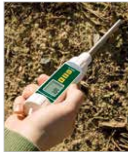
Includes 8" (20cm) stainless steel moisture probe
