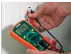
Displays AC Voltage of an outlet receptacle
