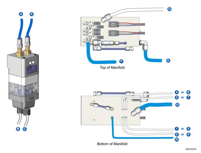
Figure 13 Air and Powder Tubing Part Numbers
