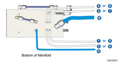
Figure 8 Powder and Air Tubing Connections
