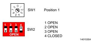
Figure 4 SW1 and SW2 Settings for a Manual Powder Spray Systems
