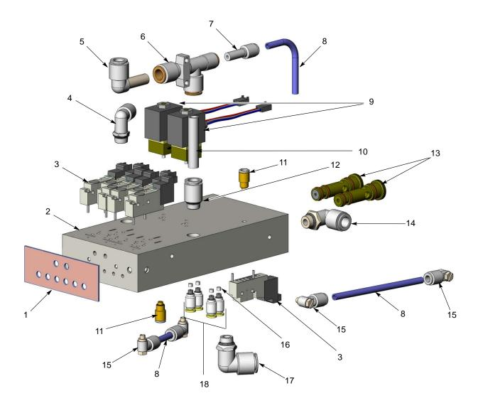
Figure 11 Manifold Parts
