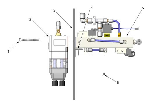
Figure 2 Pump and Manifold Installation
