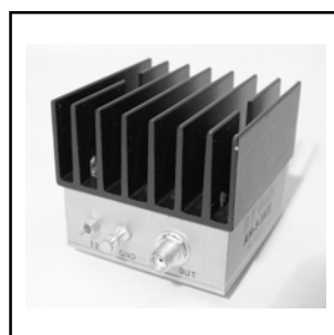
AM-5-1A12 2-500 MHz, 1W, Gain 30dB, 12.5V, Class A Price: $145.00
