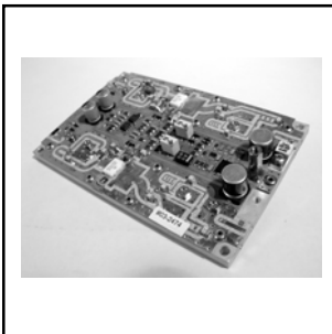
LDV75PG 134-176 MHz, LDMOS Tech., 75W CW, 60W@- 40dBC (two-tone) for PAGER applications Price: $524.00
