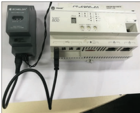
Figure 36. LON wiring, ref. 50712792
