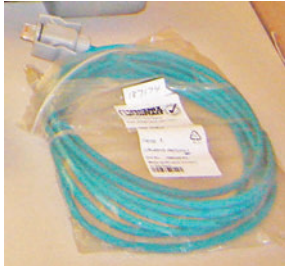
Figure 3. Wire harness extensions: M to F connectors and F connector to stripped
