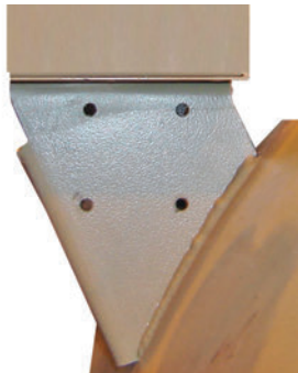
Figure 19. Display arm mounting holes drilled through right-hand panel bracket
