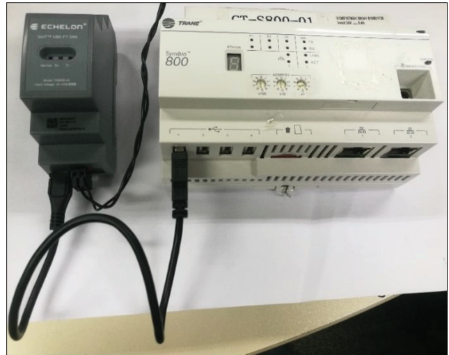
Figure 16. LON wiring, ref. 50712738
