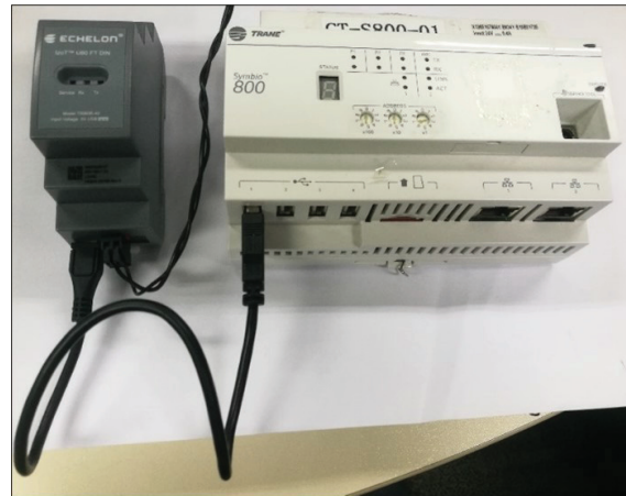
Figure 18. LON wiring, ref. 50712737
