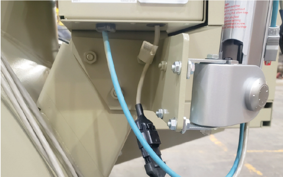
Figure 7. Bolting display arm to the panel
