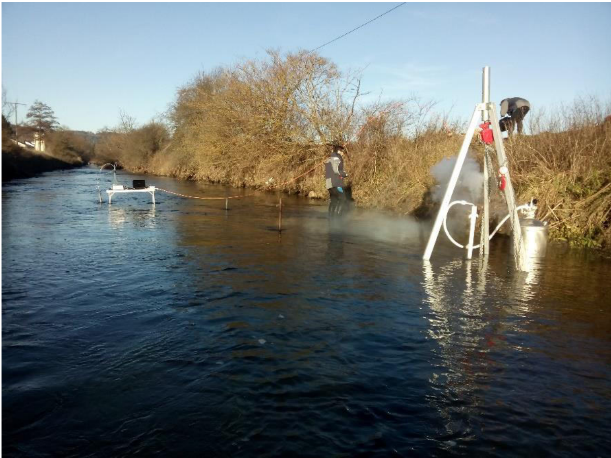
Figure 4.20: Image of River Würm including set up for the VertiCo measurements at Würm 4 and freeze-core sampling at Würm 1. Image is facing downstream direction.
