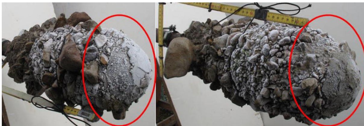
Figure 7.10: Layer with fine material at the bottom of the two sediment samples Würm 1 (left) and Würm 6 (right).
