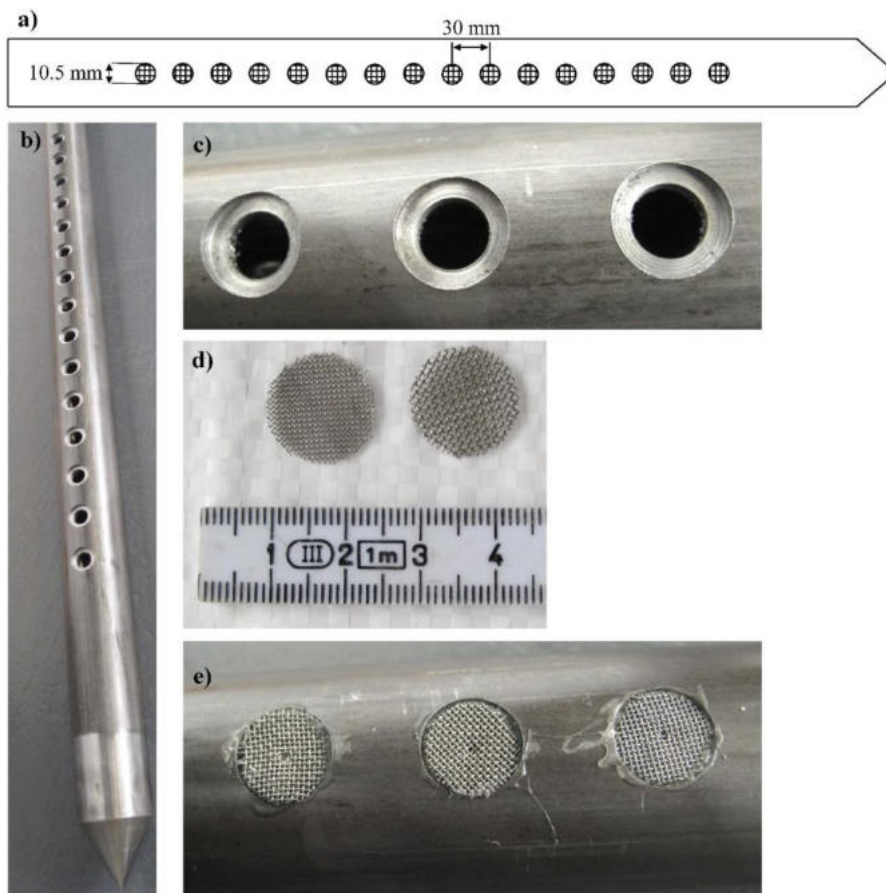
Figure 3.4: Set-up of the optimized standpipe a) schematic sketch of the standpipe b) standpipe without covering of the openings c) close up from the openings with the lowering for the mesh to be fixed d) fine mesh on the left side to prevent fine sediments to enter the standpipe and coarse mesh on the right side to protect the fine mesh from destruction e) example of glued mesh in the standpipe.
