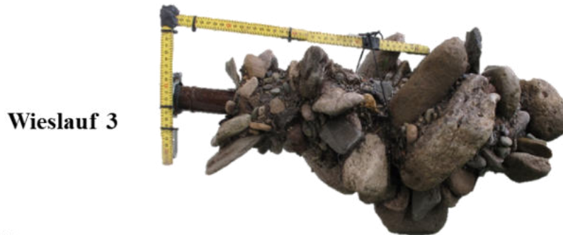
Appendix 2. 13: Results from Wieslauf 3 including image of sediment sample, cumulative sieve curve and vertical profiles from slurping rate, IDOS and kf.
