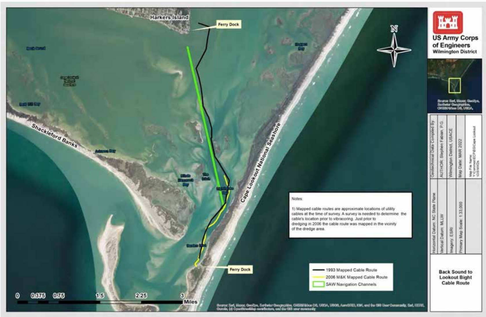
Figure 2. Mapped cable routes from Harkers Island to Cape Lookout Lighthouse. The 1993 route covers most of the cable route while the 2006 mapped cable route covers a small portion of the cable's location, which was in the vicinity of where dredging occurred 2006.
