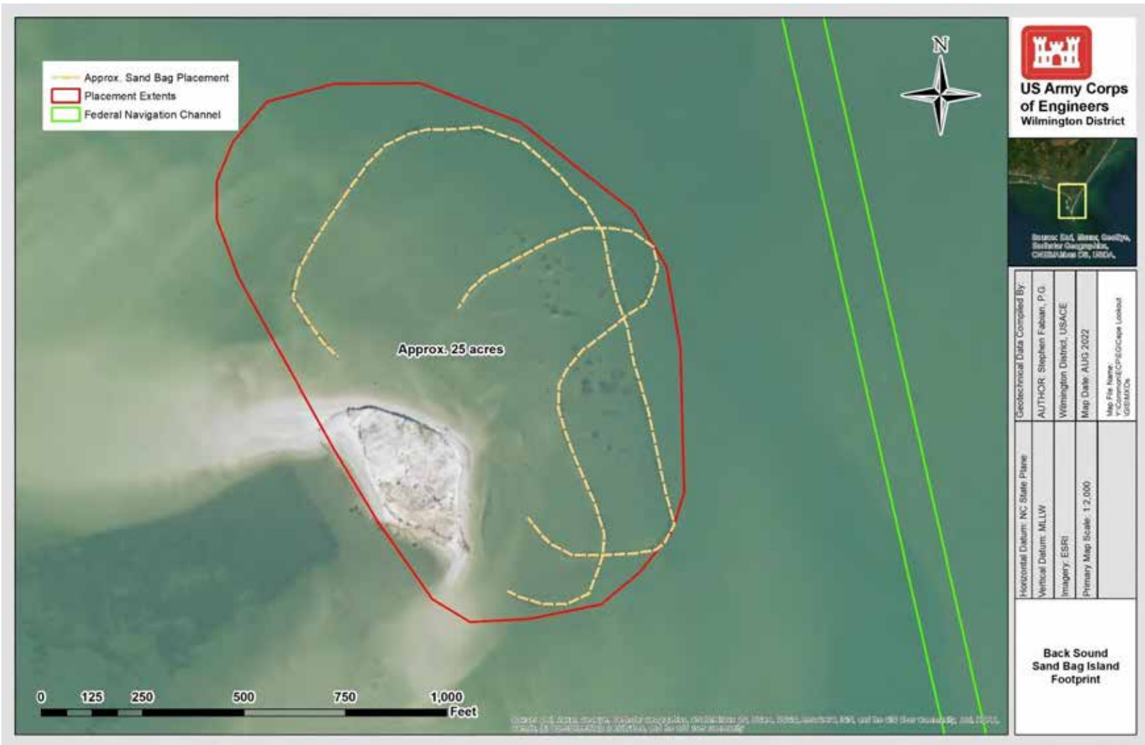
Figure 3. Sandbag Island, a bird nesting site, was last used in 1997. The island’s footprint has changed numerous times due to sediments being reworked by wind, tides, and coastal storms. Old sandbags (dashed orange line) used to control the movement of material are still visible today.
