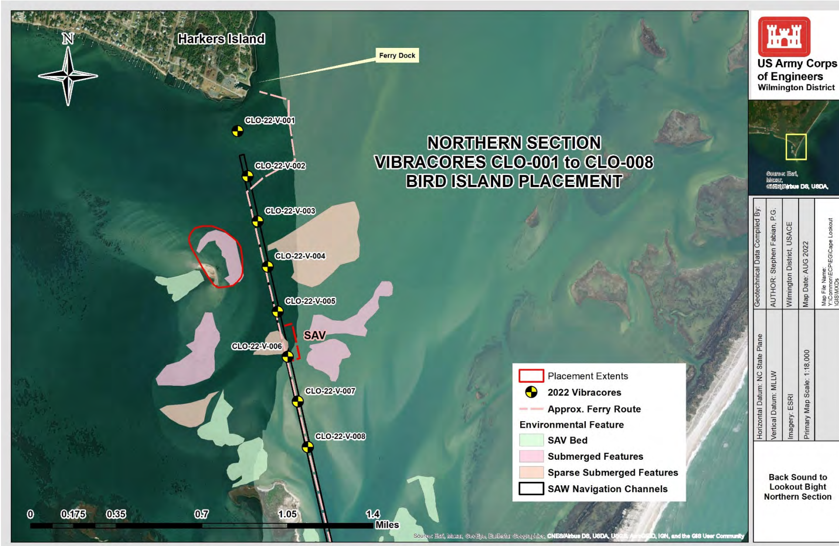
Figure 12. Showing dredging limitations within the northern section of the study area. It is recommended all material dredged within the federal navigation channel be placed on the sandbag island (red polygon).
