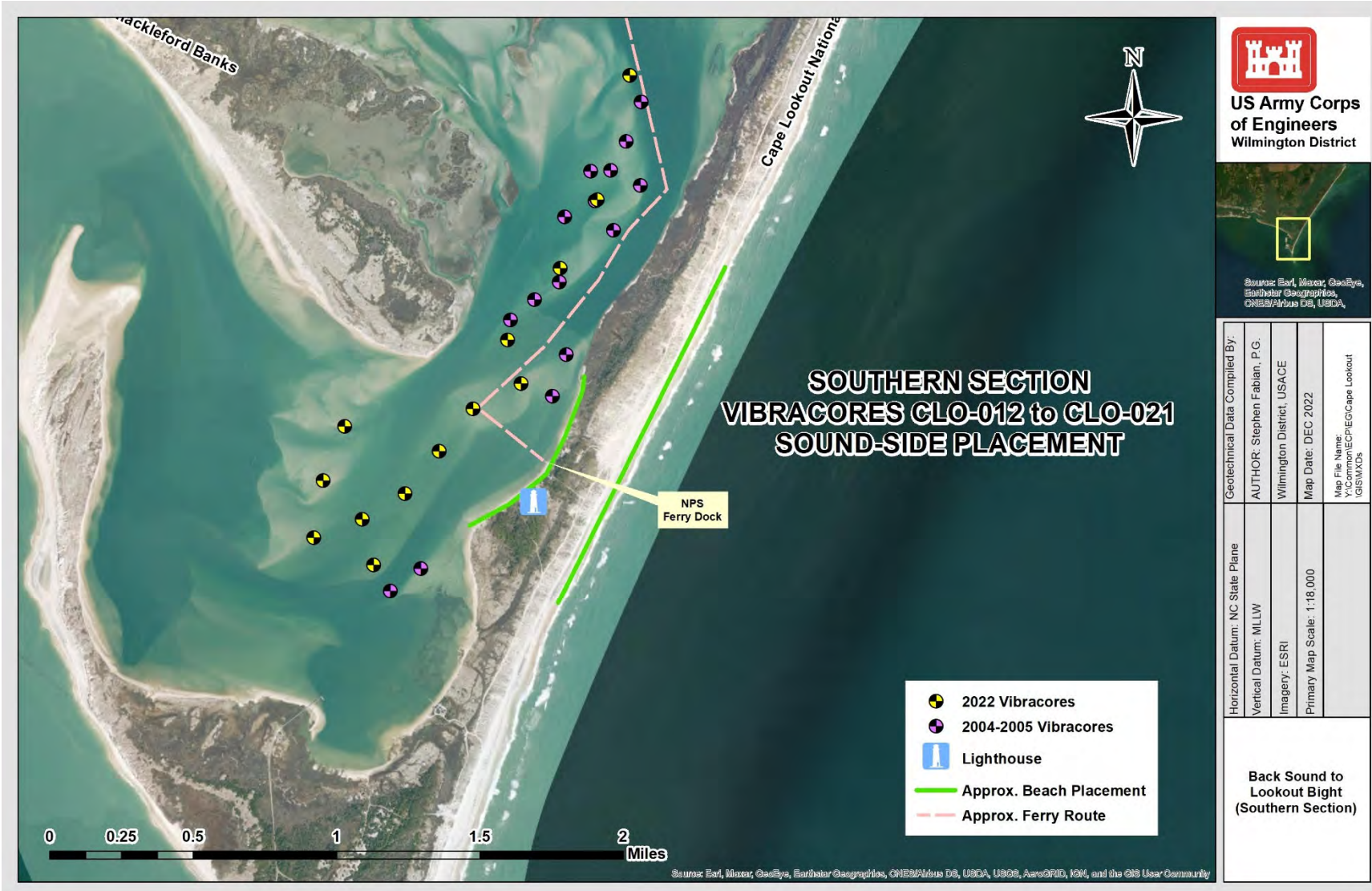
Figure 15. Vibracores collected within the southern section of the study area. It is recommended all dredged material within this area be placed on the sound-side beach in front of the Cape Lookout Lighthouse.
