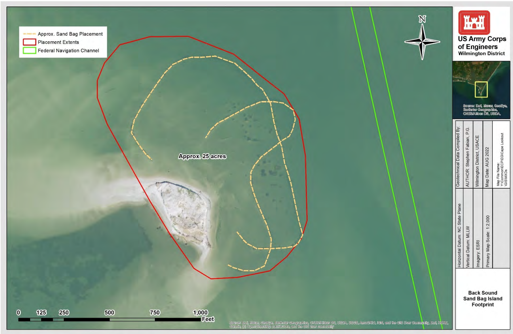
Figure 3. Sandbag island, a disposal site, was last used in 1997. The island's footprint has changed numerous times due sediments being reworked by wind, tides, and coastal storms. The sandbag ring (dashed red line) used to control the movement of material is still visible today.
