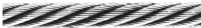
Left Regular Lay – Strands are laid to the left and wires appear in line with the rope.
