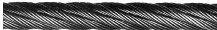
Right Lang Lay – Strands are laid to the right but the wires appear to make an angle with the rope.
