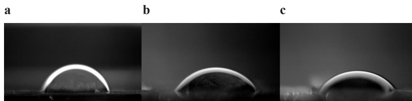
Figure 1. Water contact angle and wettability. a Large wetting angle: hydrophobic surface (untreated PVDF+ \text{CoFe}_2\text{O}_4 sample). b , c Small wetting angle: hydrophilic surface (PVDF+ \text{CoFe}_2\text{O}_4 samples treated for 60 and 90 seconds respectively).
