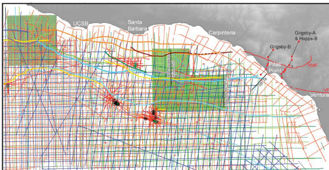
Figure 5. Part of the basemap of 2D MCS lines and 3D seismic surveys (green grids) used to correlate and map offshore faults, folds and stratigraphic reference horizons in 3D (e.g., Fig.4 ) [Sorlien et al. , 2014; Sorlien and Nicholson, 2015]. Also shown are tip lines or surface traces of mapped faults and the well locations used to construct the correlation cross sections near Pitas Point (e.g., Figs.2&8 ) [Grigsby, 1988; Hopps et al. , 1992].
