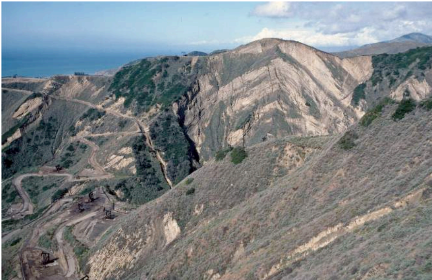
Figure 10. This is NOT the Ventura Avenue anticline! It is the distinctly separate San Miguelito anticline! This classic amphitheatre photo looking west is often mistaken for the Ventura Avenue anticline [e.g., Rockwell, 2011], which is located below and farther east along trend. However, this is the asymmetrical N-verging San Miguelito anticline and oilfield. Pitas Point is located at the coast just off the photo at left. Photo credit Art Sylvester.
