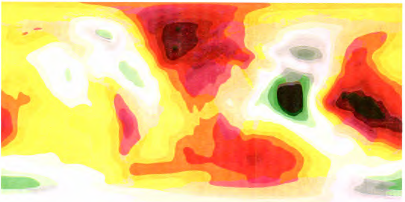
Figure 2.14. The ERS-1 gravitational equipotential model showing with coloured isocontours the range -105 m (blue) to 85 m (red). The gravitational geopotential produces the principal acceleration on the Earth. A precise orbit restitution applying dynamic methods therefore requires a precise model of the geopotential, with resolution requirements depending on the satellite's altitude.
