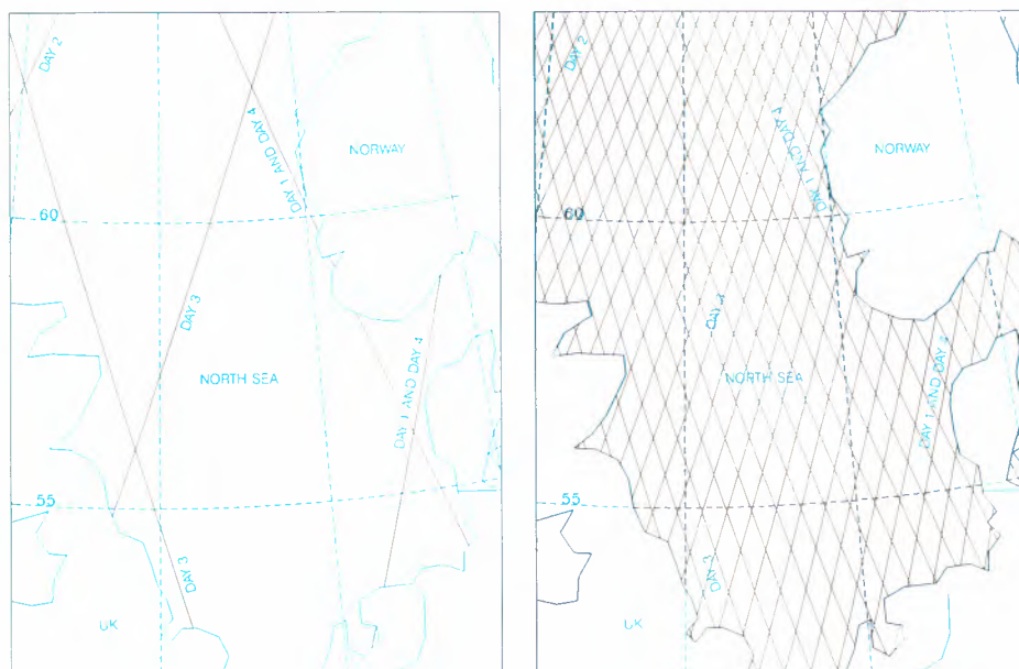
Figure 1.2. A comparison of the density of Radar Altimeter tracks over the North Sea using 3-day and 35-day repeat cycles.
