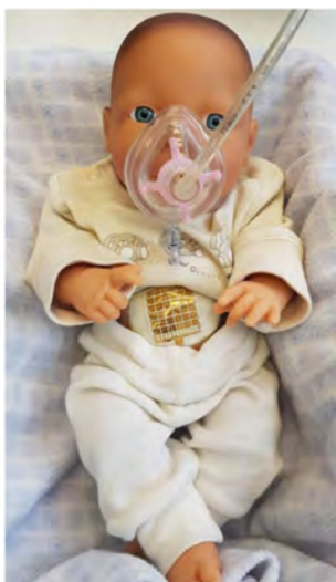
FIGURE 2: Sensorpatch attached to a dummy Shown is one of the configurations used for in-vitro testing.
