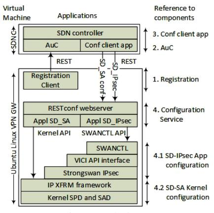
Fig. 8. Components in the architecture.
