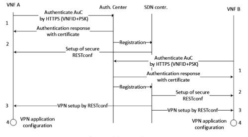
Fig. 5. Detailed sequence diagram.
