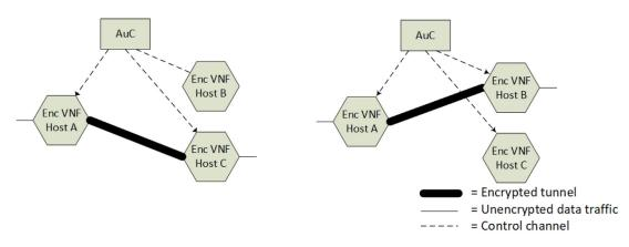
Fig. 3. The dynamic behaviour of VPN tunnels.
