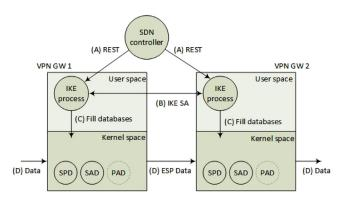
**Fig. 6.** Updating IPsec configuration by RESTconf and making a Security Association (SA) by using IKE.
