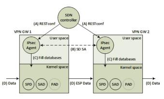
**Fig. 7.** Distributing keys directly from controller by RESTconf and making a Software Defined Security Association (SD-SA).
