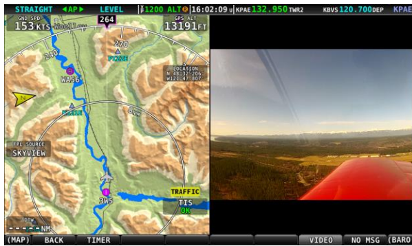
Figure 230 – Half Screen Map/Video Display
