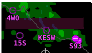
Figure 165 – Missing NEXAD Data Blocks
