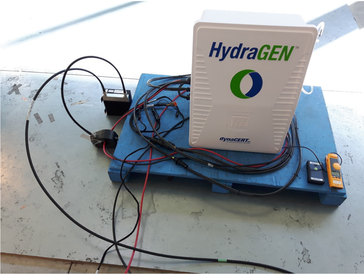
Figure 6 – Conducted Immunity Setup
