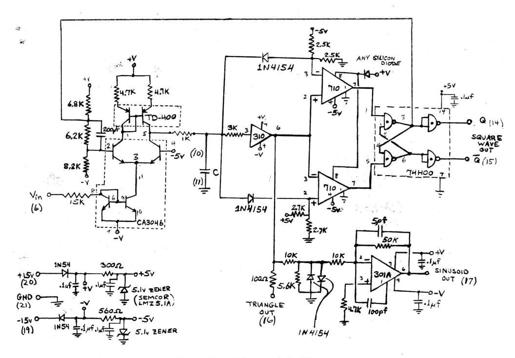
Fig. 1: Circuit Diagram of the VCO
