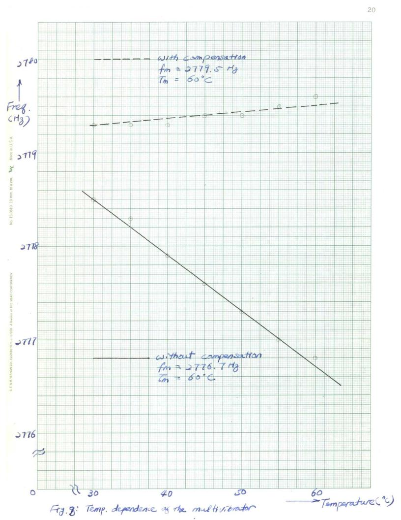
multivibrator has S of 0.00024 %/C. The improvement is by a factor of 9 and the design objective of low cost has been met while that of the frequency stability coefficient has been surpassed.
