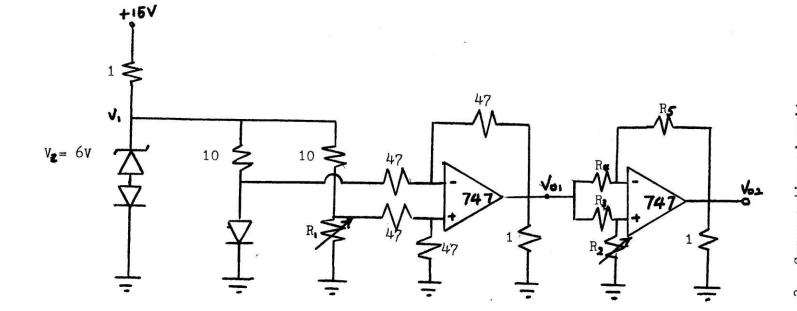
All resistances in KO  $R_{1} = 1$  KO  $R_{2} = 10$  KO  $R_{3} = R_{4} = R_{5} = 2$  KO  $\mathbb{P}^{1}\mathcal{E}$ . 3: Compensation circuit
