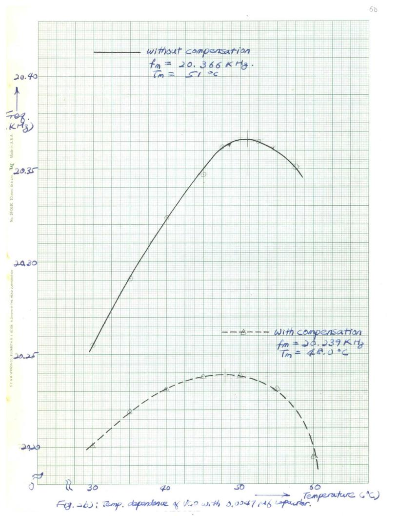
capacitor of the VCO. Tables 1(a) and 1(b) are plotted in Figs. 2(a) and 2(b). As can be seen from the Figs. 2(a) and 2(b), the frequency dependence on the temperature is not linear but the curve is continuous and differentiable. Therefore, this dependence can be expressed in a Taylor series. The linear compensation scheme would neutralize the linear part of the Taylor series but it would have no effect on the other parts of the series. Still, this could be a significant improvement.
