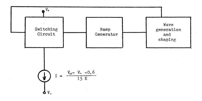
Fig. 5: Block diagram of the VCO
