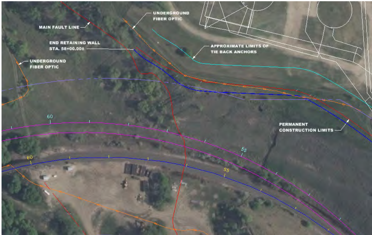
Figure 7 – Wall Location 2 Utility Conflicts
