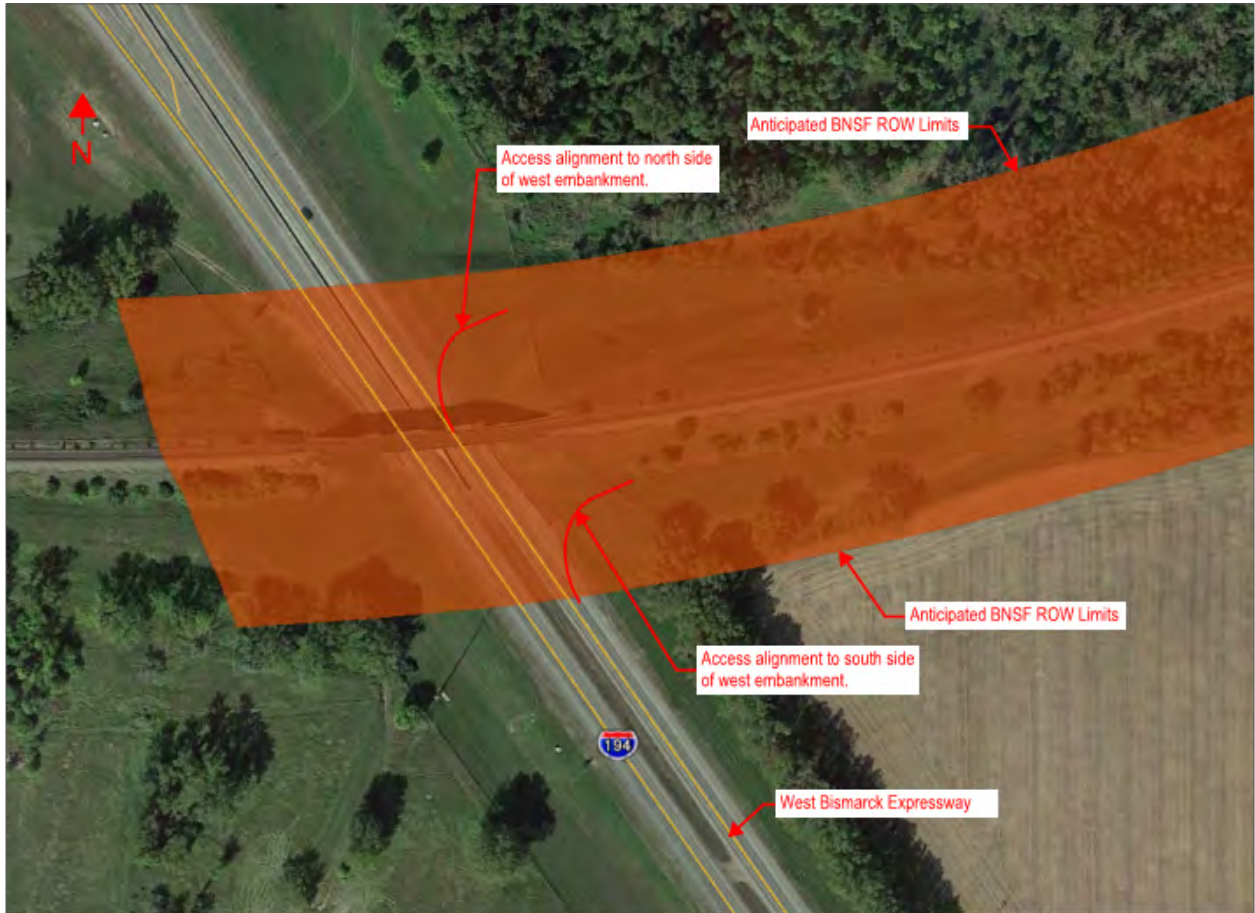
Figure 18-3. West Approach Access
