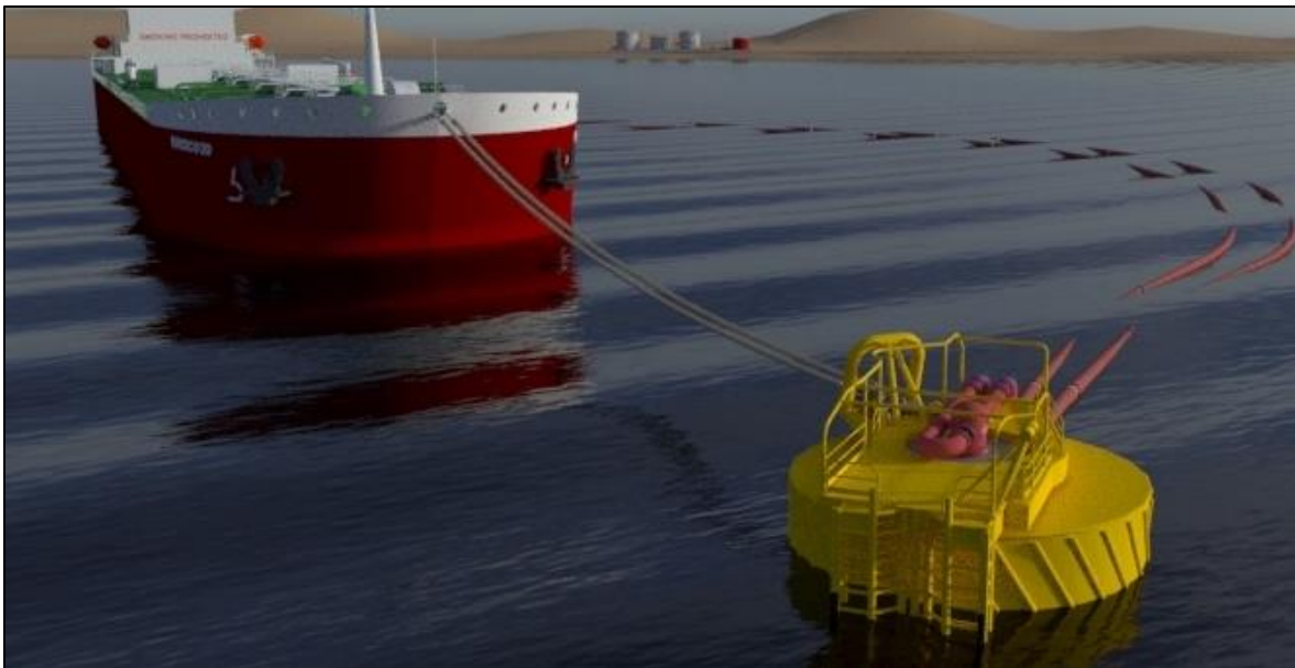
Figure 18. Above-water Depiction of a Tanker Moored at a SPM CALM Buoy
